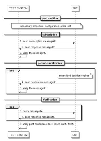
Figure 4.5.3.3.2-1: Verification procedure
