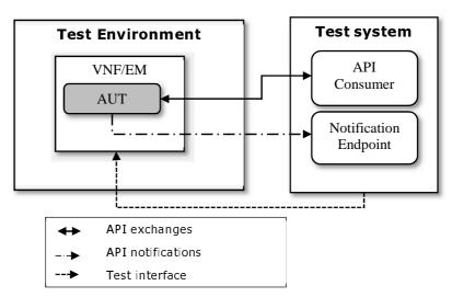
Figure 4.3.2-1: Configuration for tests of APIs with the FUTs as Producer run in a VNF/EM
