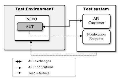
Figure 4.3.4-1: Configuration for tests of APIs with NFVO as Producer
