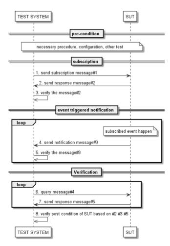
Figure 4.5.3.3.1-1: Verification procedure
